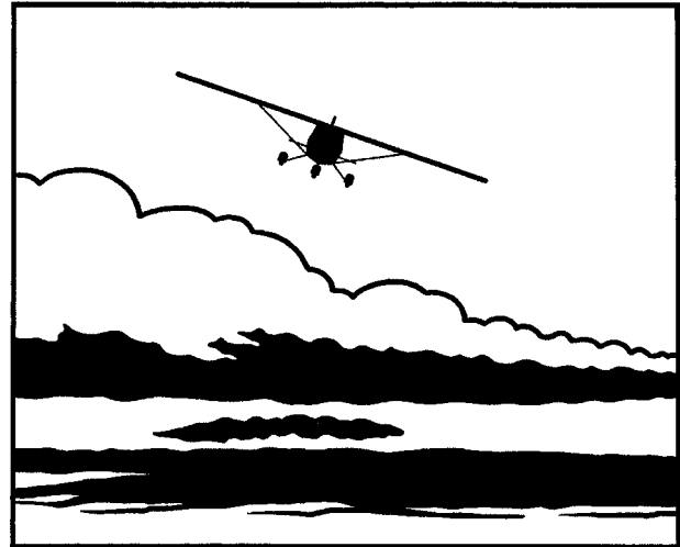
FIGURE 6-22 A sloping cloud deck, which the pilot misperceives as a horizontal surface.
