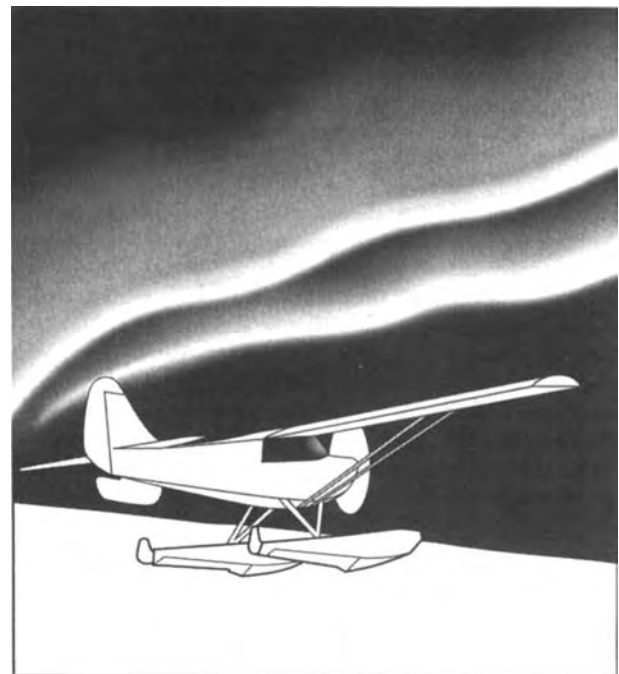
FIGURE 6-23 Aurora Borealis appears as a false horizon. As aurora curtain shifts, pilot attempts to follow the false horizon.
